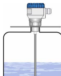
Fig. 6: Incorrect welding flange mounting to the tank
